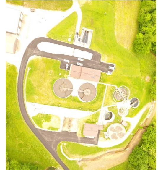
In 1984, the plant capacity was expanded to 700,000 gallons per day, an oxidation ditch installed, 2 clarifiers, a sludge holding tank, and a vacuum sludge drying building were added. Sewer mains were extended to a subdivision of 154 lots near the lake, a recreational campground with 700 lots and extensions to connect across the lake to a proposed commercial development (Tillery Hill). Total cost was \$2.2 million.
